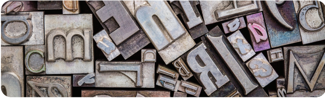
Backwards letters on old metal printing blocks, which were arranged into words on a printing press.
